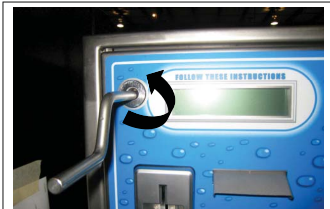
Lock Wrench in Unlock Direction
